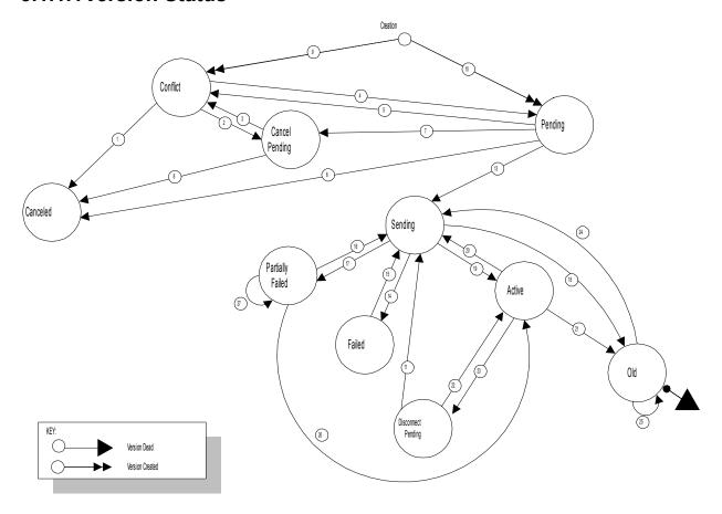
Figure 5-14 Version Status Interaction Diagram
